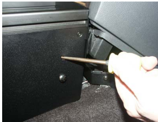
Attach main console housing to previously installed floor bracket using 1/4" carriage bolts and nylock nuts. Use a scribe or awl to help align (7/16" socket, awl)
